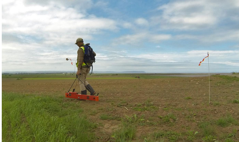
Figure 1. Conductivity survey with Geonics EM38Mk2, Grand-Pré, Nova Scotia
