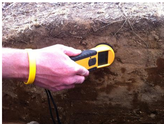
Figure 6. Collecting field magnetic susceptibility readings using the handheld Terraplus, Inc. KT-10.
