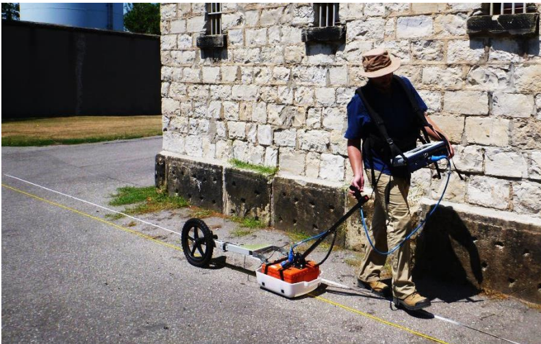
Photo: GPR analysis in progress (c/o Timmins Martelle Heritage Consultants, Inc.)
